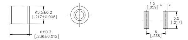
**Recommended Soldering Pad Layout**
